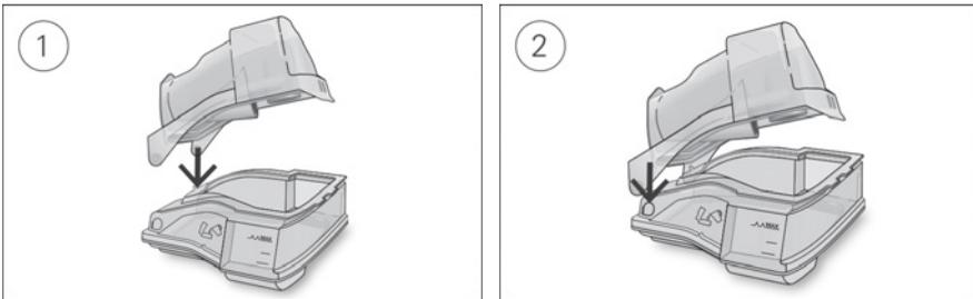
1. Insert one side of the lid into the pivot hole of the base.
