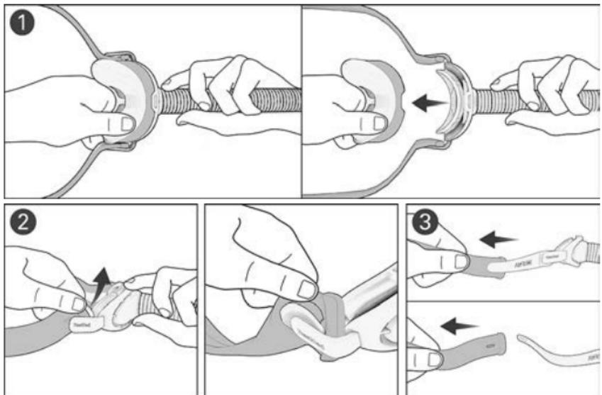
1. Firmly pinch one side of the cushion and pull away from the frame.
