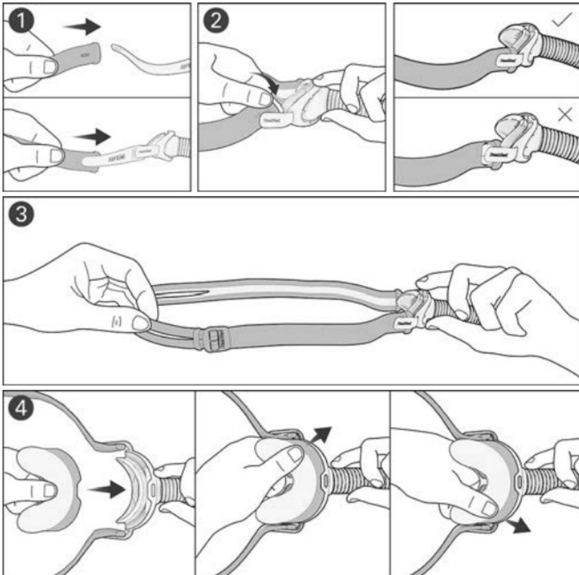
1. With the grey side of the headgear facing out, insert each end of the headgear band over the stabilisers through the buttonholes.
